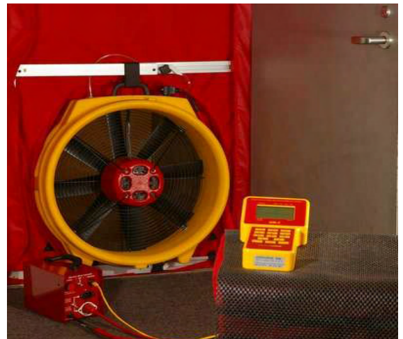
Picture of Air Pressure Testing Equipment used by our organisation.
